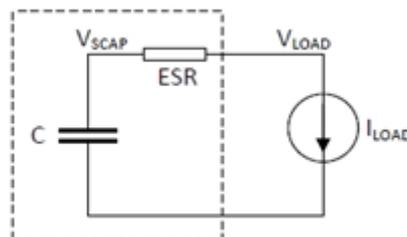
Figure 9. Ideal Super Capacitor model with series ESR.
