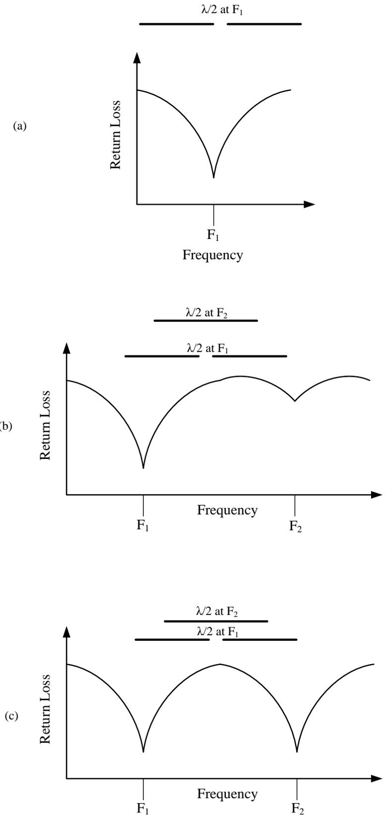
Figure 2. (a) Return loss plot of a dipole over a wide frequency range. At (b) a nearby conductor is just close enough to interact with the dipole. At (c) the second conductor is at optimum spacing. The combination is matched at both frequencies.
