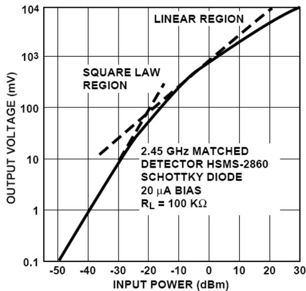
Figure 8. Detector transfer curve.
