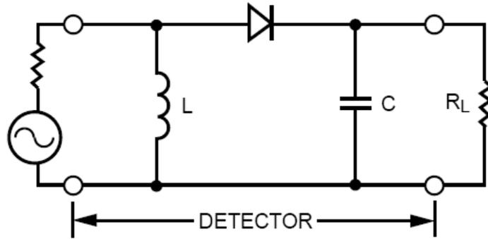
Figure 7. Diode detector.
