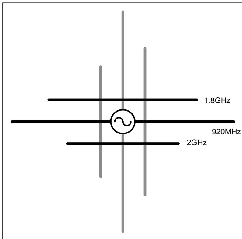
Figure 3. Three band GSM energy harvesting antenna. Both horizontal and vertical elements are placed on opposite sides of the supporting substrate.
