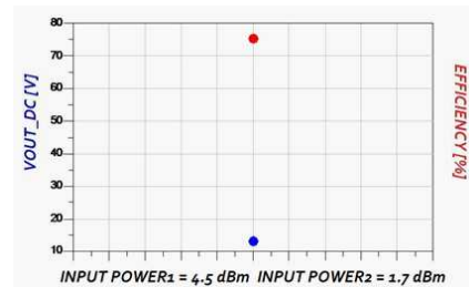
Figure 13. Co-simulation results: output voltage and efficiency rectification of the 900 MHz–2.4 GHz rectenna when the RF input power1 (900 MHz) is 4.5 dBm and the RF input power 2 (2.4 GHz) is 1.7 dBm.
