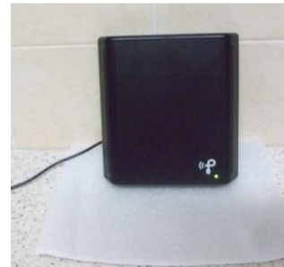
Fig2 (a), a side view, and (b) a real view of a TX91501 Powercaster Transmitter in its transmission state
